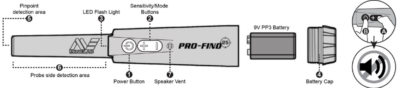
To turn the PRO-FIND 25 on, make sure there are no metal objects nearby (at least 300 mm/12 in) and press and release the **Power Button (1)**. The unit will beep twice and the **LED Flash Light (3)** will illuminate. A further short beep will sound when the unit is ready to use.
